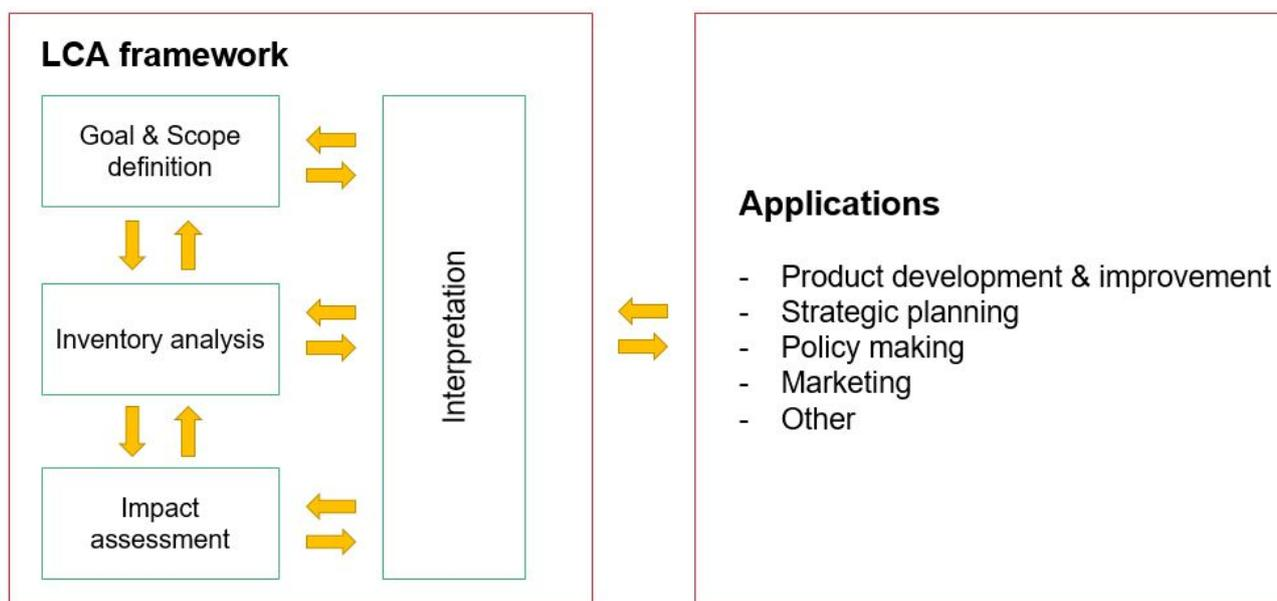
Figure 1: ISO standard based framework for LCA
